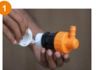
Start winding some PTFE sealing tape on the outside of the threaded male end, taking care not to obstruct the through-hole on the pipe, fitting or valve Complete the first winding layer by winding the tape clockwise until you reach theroot of the thread.
