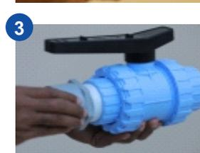
Ensure that the tape adheres completely to the male thread. Connect the previously sealed male end to the female end and proceed manually by screwing the two elements
