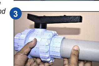
Fully insert the pipe into the fitting immediately and without any rotation as soon as possible
