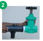
Connect the previously sealed male end to the female end and proceed manually by screwing the two elements
