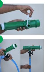
Complete the first winding layer by winding the tape clockwise until vou reach the root of the thread.
